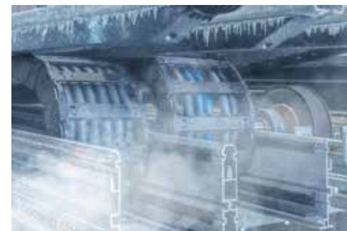
Climate chamber. Dynamic tests of cables in e-chains® at -40°C
