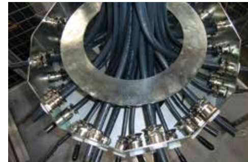
Testing of chainflex® cables under torsion
