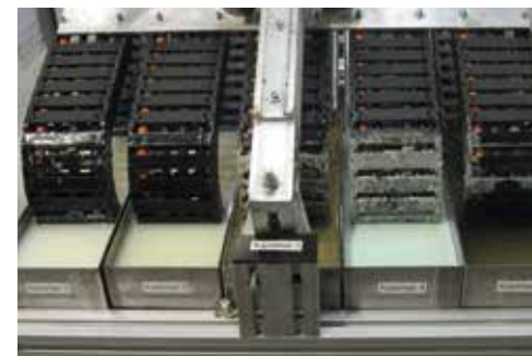
Durability test in various oils and liquids
