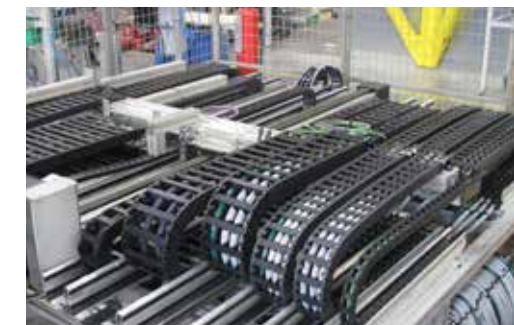
Continuous motion tests with defined bend radius
