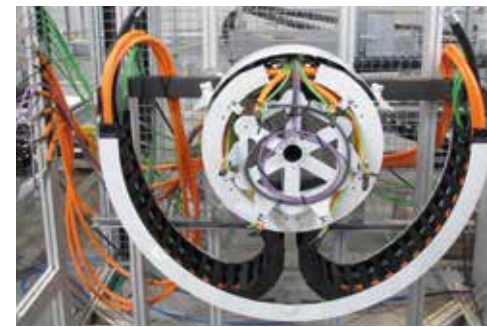
Service life test for circular movement
